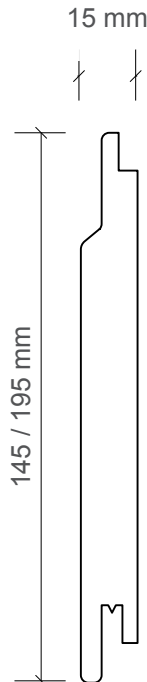
James Latham LT AC 01 tongue and groove profile for horizontal cladding
